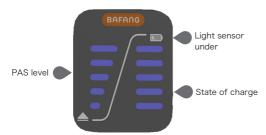
• State of charge indication: 5 LED indicate the state of charge, if the lowest LED flickers, it means the time to charge the battery
